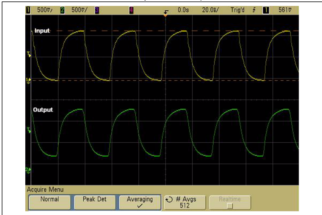
Figure 32. Sine wave input clock vs. output clock (STCD1040, 1.8 V version, 26 MHz sine wave master clock input from TCXO)
